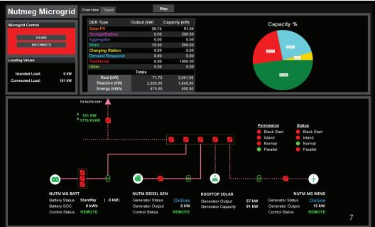
power flow, DERMS allows operators to analyze the impact of DERs on the grid, to create alarms that warn when DERs are causing issues, and—in some cases—to control how they operate by shutting them down or curtailing operation to
