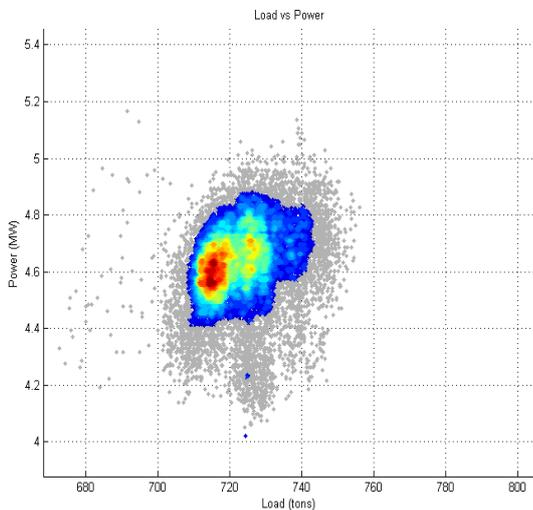
**Figure 9:** Power vs. Load density plot for periods with the MPC optimization in control.
