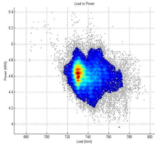
**Figure 8:** Power vs. Load density plot for periods with only fuzzy rules-based control active before MPC optimization.
