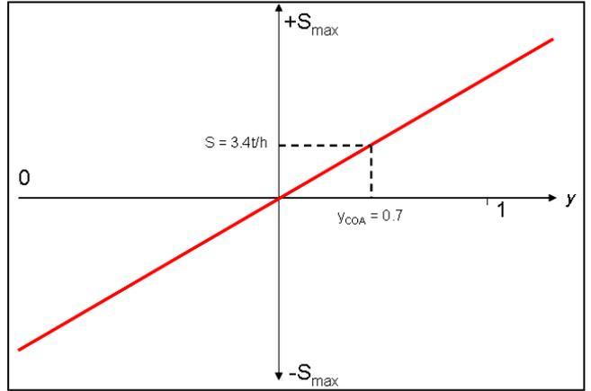
**Figure 6:** Defuzzyfication resulting in a positive mill feed step of  $S = 3.4t/h$ .
