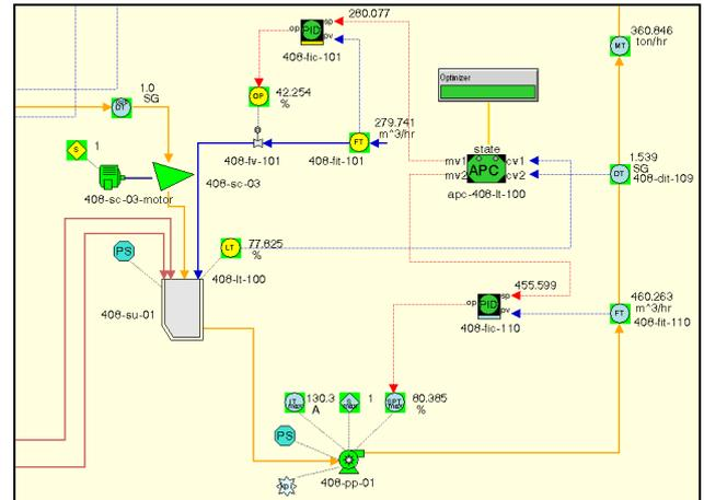
**Figure 3:** APET control schema for the primary ROM ball mill discharge sump circuit.
