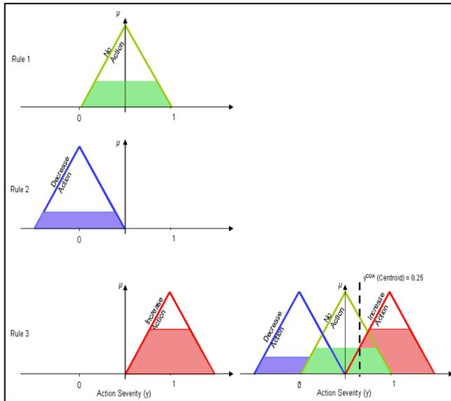
**Figure 5:** Combining the rules by means of the Centre of Area method
