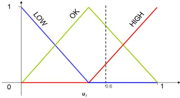
**Figure 4:** The fuzzy membership function of the normalized mill load ( $u$  on  $x$ -axis) with three membership functions (LOW, OK and HIGH).
