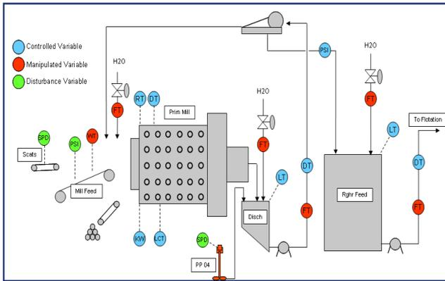
**Figure 1:** Process flow diagram of the primary ROM ball milling circuit.
