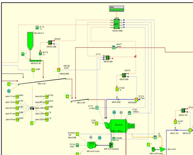
**Figure 2:** APET control schema for a primary ROM ball mill.
