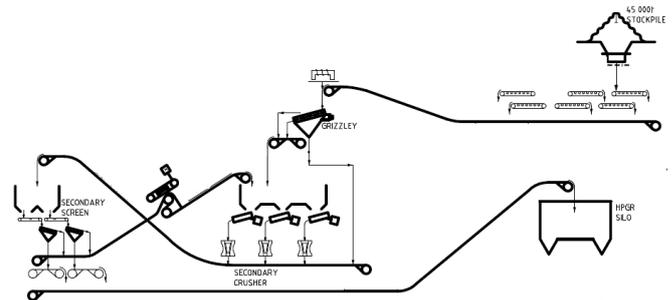
**Figure 1:** A typical Anglo Platinum secondary crusher circuit process flow diagram (PFD).
