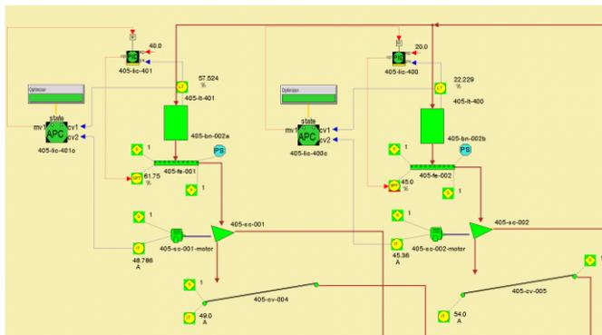
**Figure 3:** Example of a screen bin APC in APET that manipulates the screen feeder speed to control the bin level and prevent a screen overload.
