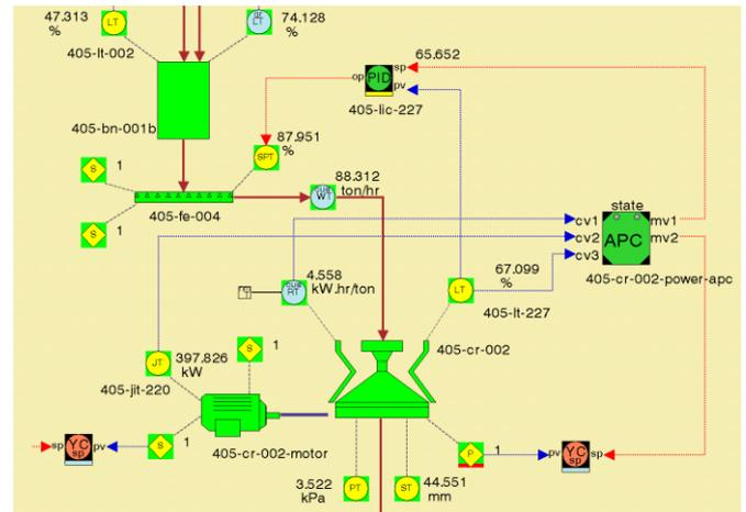
**Figure 4:** Example of a cone crusher APC in APET that manipulates the crusher cavity level PID SP and crusher closed side setting (ASRi controller) to control the crusher power draw.
