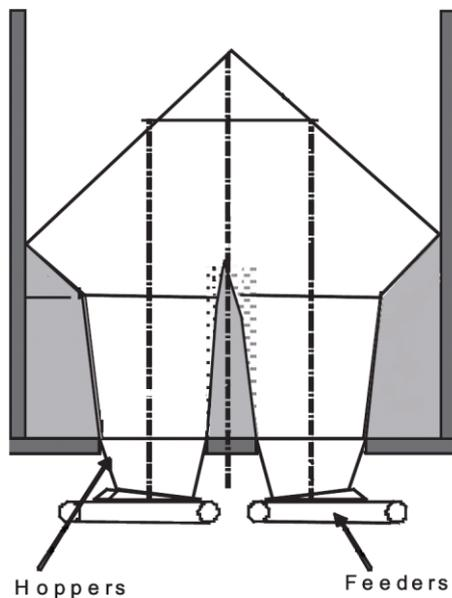
**Figure 5:** Funnel flow of material build up inside the secondary screen feed bin
