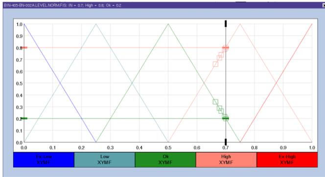
**Figure 2:** Fuzzy membership functions showing the functions, overlaid with recent data, used to fuzzify the bin level.
