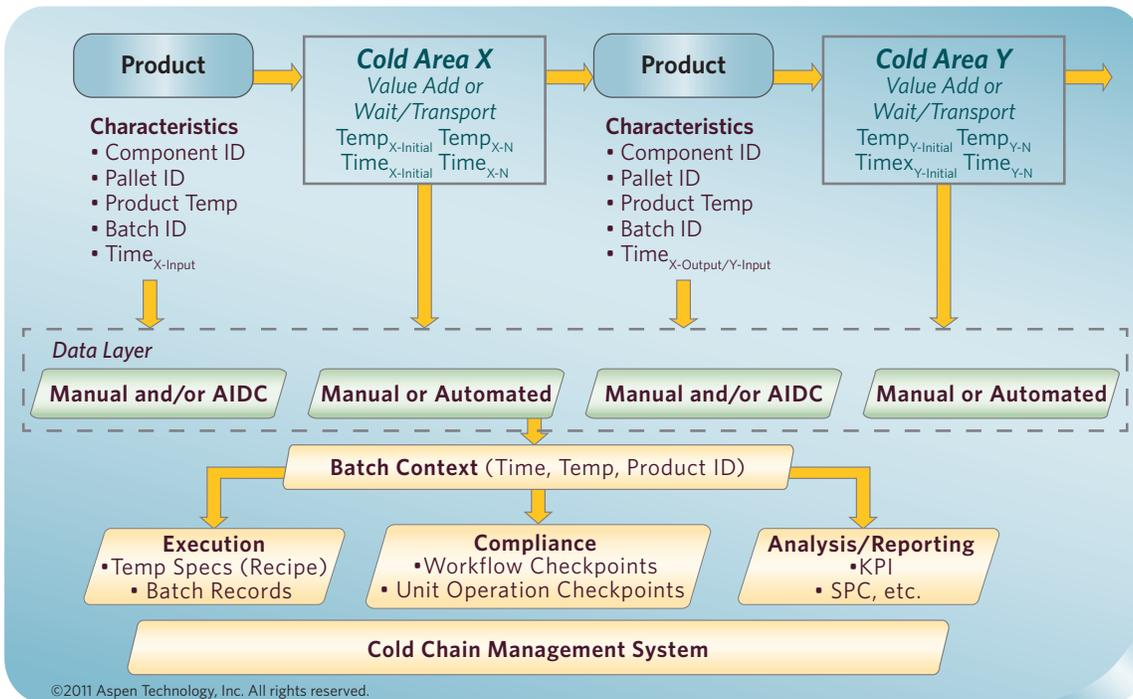
Figure 1: Example of an in-facility Cold Chain Management System.
